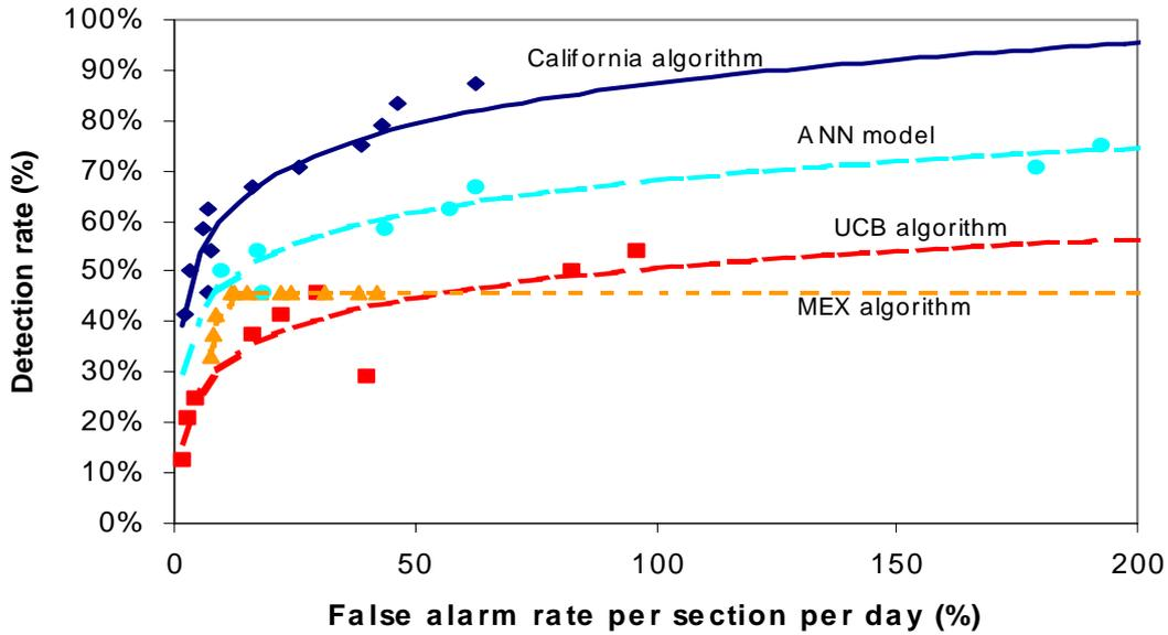
Fig. seq Fig. ¥\* Arabic 10 - Performance curves of the four incident detection algorithms
