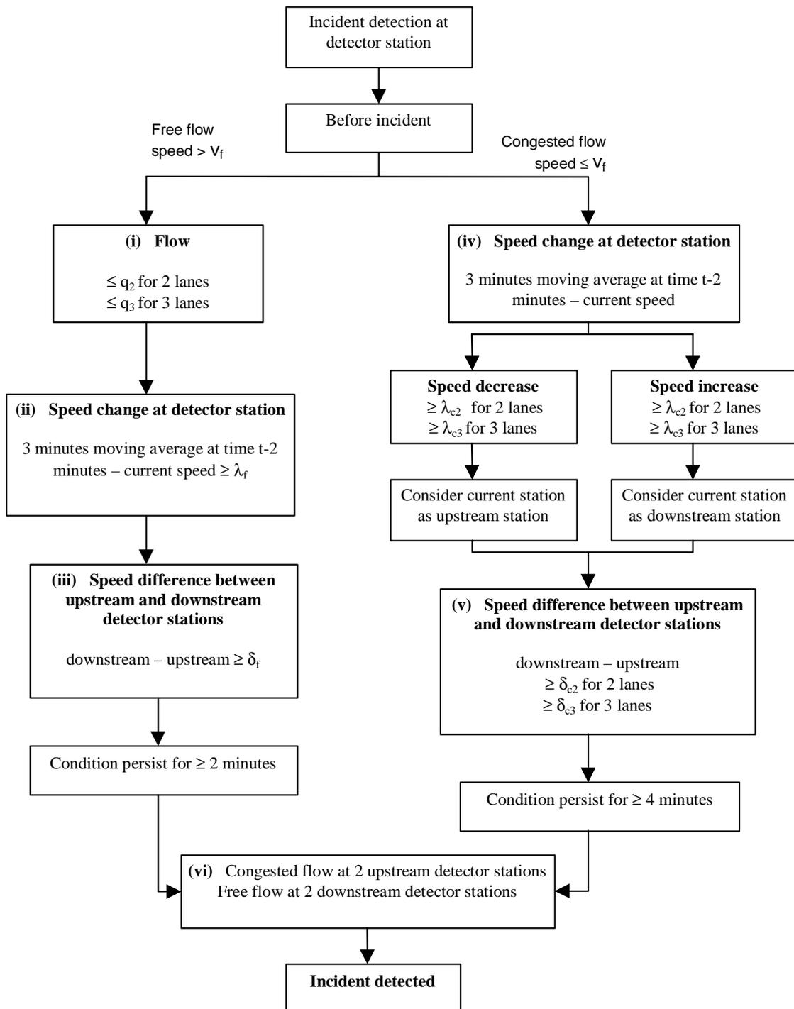
Fig. 2 – MEX incident detection algorithm flow chart
