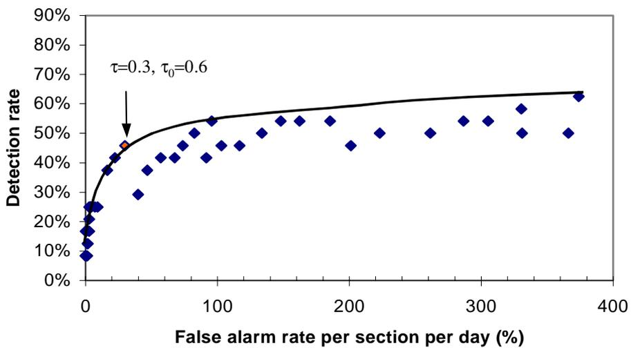
Fig. seq Fig. ¥\* Arabic 7 – Performance curve of University of California, Berkeley algorithm
