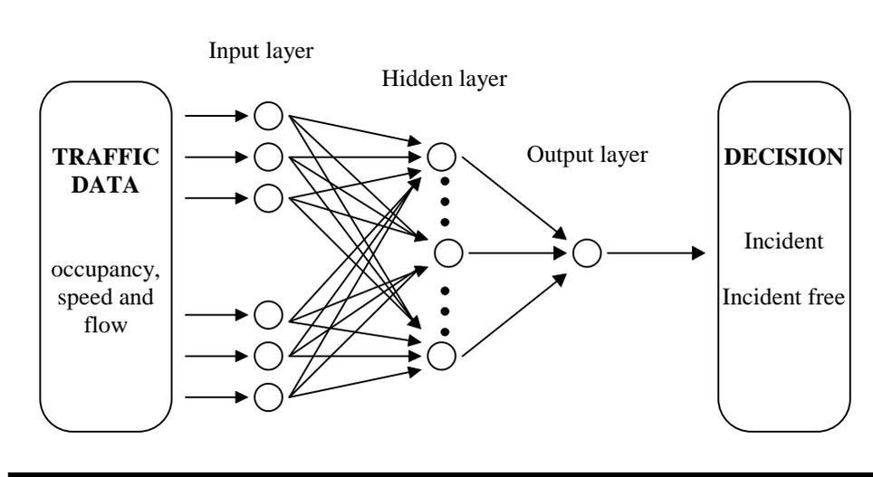
Fig. 3 - Artificial neural network modelling framework
