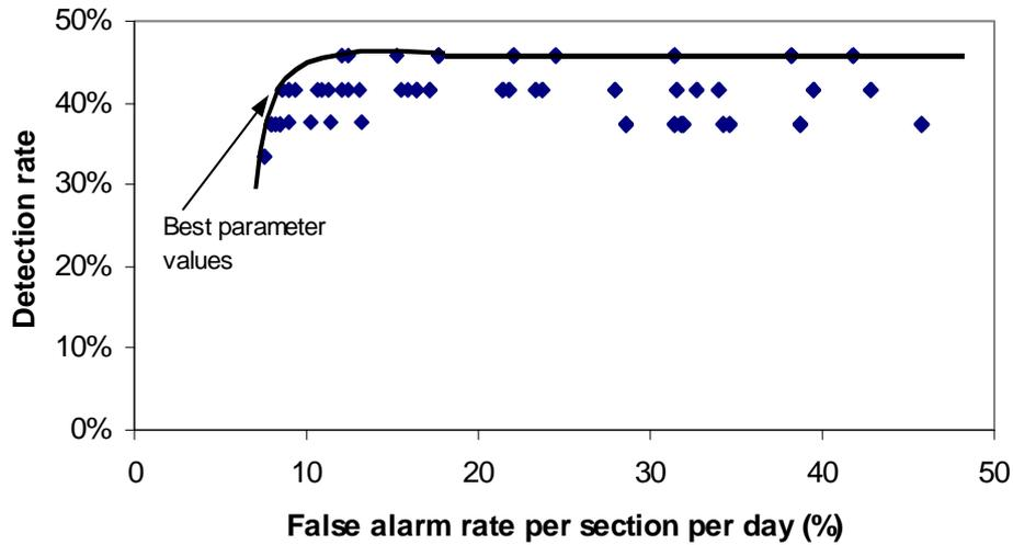
Fig. seq Fig. ¥\* Arabic 8 – Performance curve of Tokyo Metropolitan Expressway algorithm
