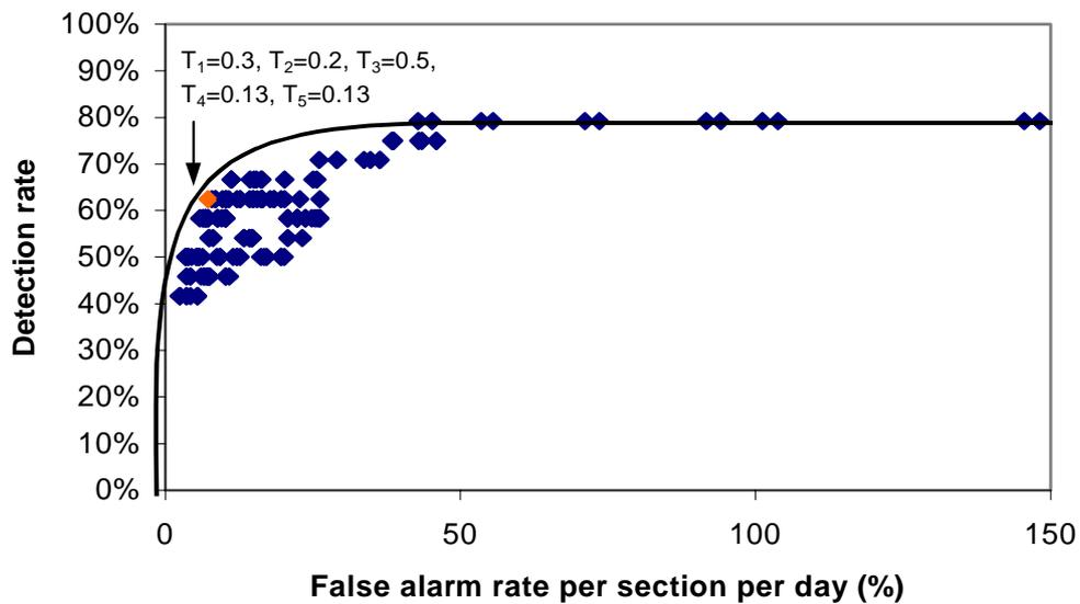
Fig. seq Fig. ¥\* Arabic 6 – Performance curve of California algorithm 8
