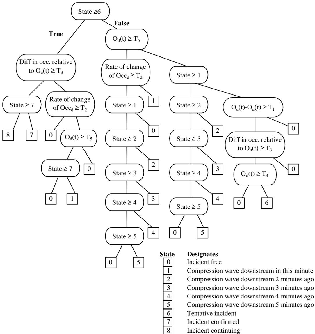
Fig. 1 - California algorithm #8 flow chart (Source: ???)
