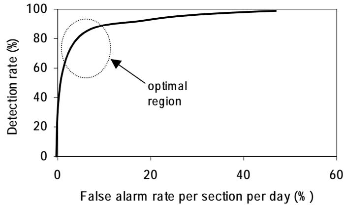
Fig. seq Fig. ¥\* Arabic 5 – Typical performance curve of an incident detection algorithm
