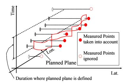
Figure 5: How to calculate distance between measured paths and planned plane
