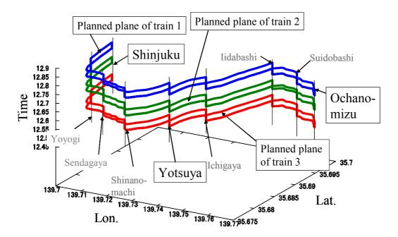
Figure 10: Example of planned path between Ochanomizu and Shinjuku
