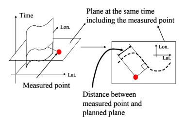
Figure 4: Definition of distance between measured point and planned plane
