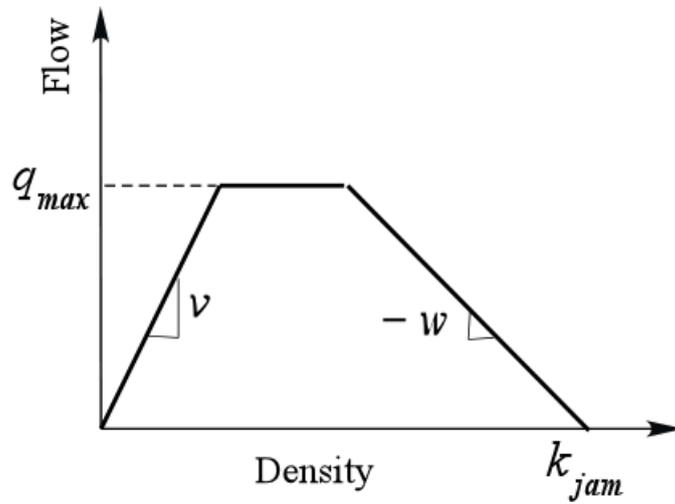
**Figure 1** Flow-density relationship for the cell-transmission model
