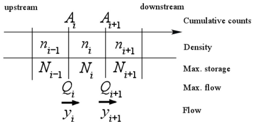
**Figure 3** State variables and parameters in each cell
