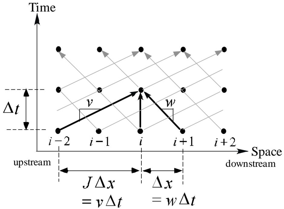
**Figure 4** Characteristic curves on a space-time grid for the cumulative count based cell transmission model (the case of  $J = v/w = 2$ )
